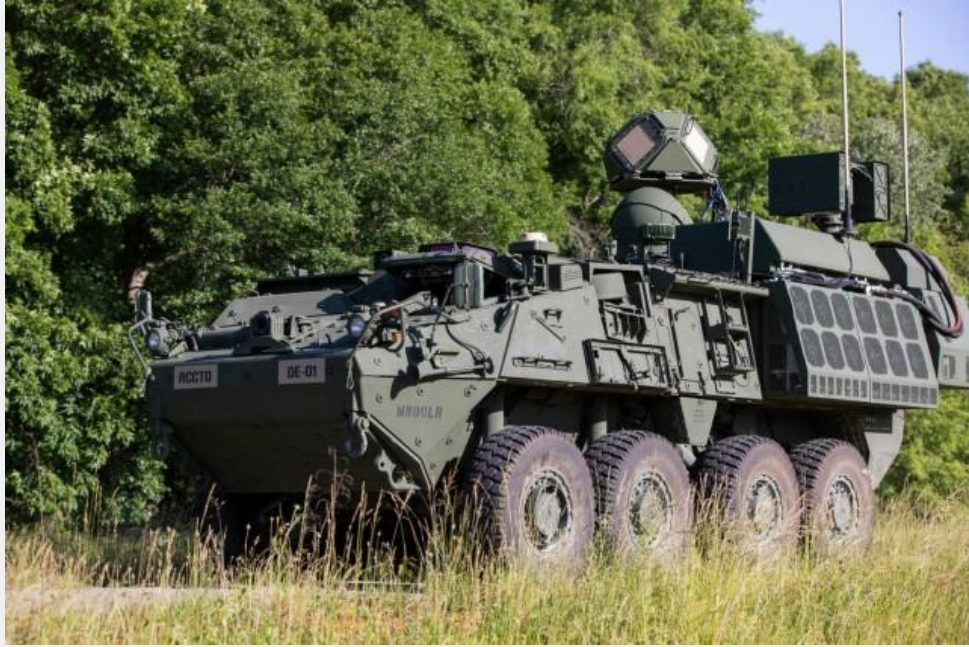
Figure 1: Directed Energy Maneuver Short-Range Air Defense (DE M-SHORAD) 50 kW-class laser weapon system mounted on a Stryker A1 8×8 armored vehicle.
